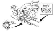
Make sure that the edges of the cutting links are facing forward on the top edge of the bar.
